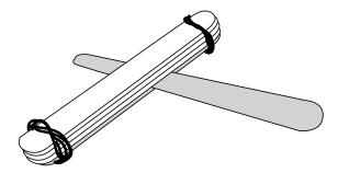
4. Put another stick on top. Use a rubber band to connect it to the shorter end of the lower stick.
