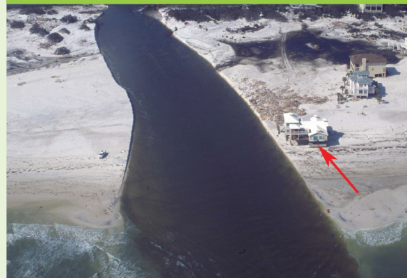
After the hurricane: Waves and storm surge have split the island in two.
