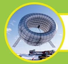
The BAT (Buoyant Airborne Turbine) is a wind turbine set inside a giant tube-shaped balloon. The balloon carries the turbine up to 610 meters (2,000 ft) high, where the wind is stronger and steadier than winds near the ground. It can be set up in less than 24 hours. That would make it good for bringing energy to disaster areas where regular power has shut down.
