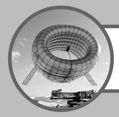
The BAT (Buoyant Airborne Turbine) is a wind turbine set inside a giant tube-shaped balloon. The balloon carries the turbine up to 610 meters (2,000 ft) high, where the wind is stronger and steadier than winds near the ground. It can be set up in less than 24 hours. That would make it good for bringing energy to disaster areas where regular power has shut down.
