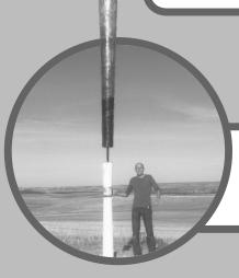
The Vortex doesn't spin at all. Instead, it sways like a tree branch in the wind. It doesn't capture as much wind power as a turbine. But its inventor says that because the Vortex has fewer moving parts, it would be cheaper to build and maintain than a turbine.
